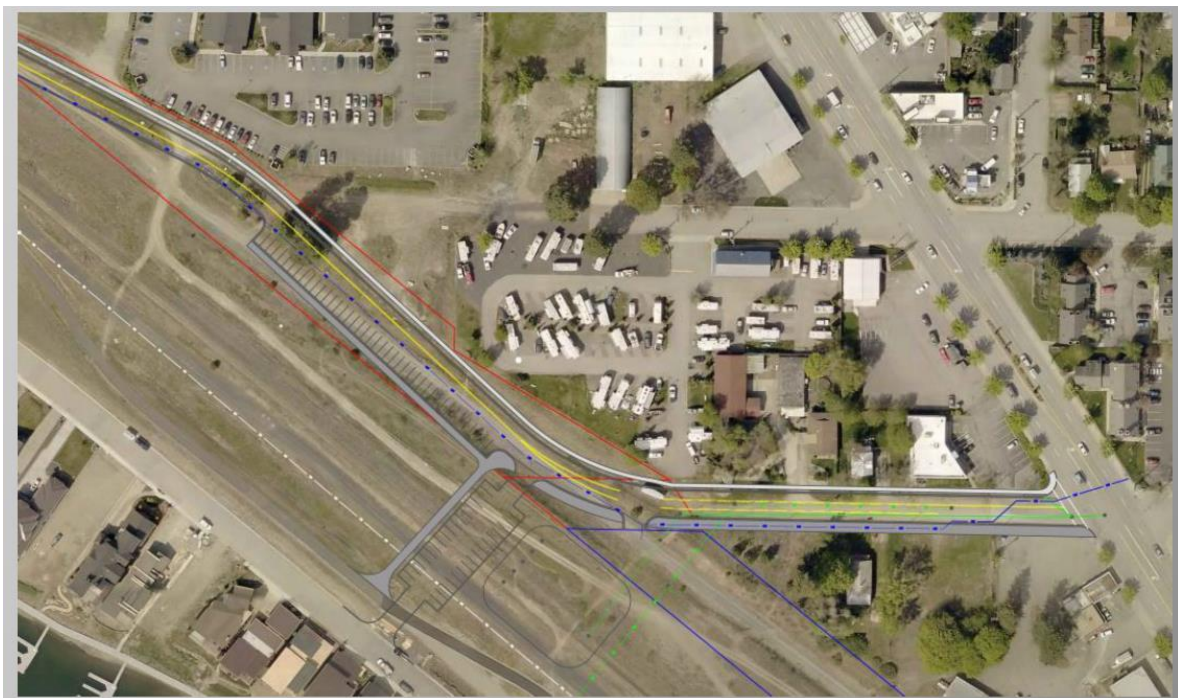
Close up view of project highlighting LaCrosse Avenue extension and proposed Bellerive connection, including new public parking areas and trails/sidewalks as depicted.
